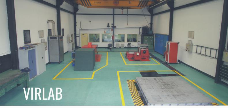
Vibration and shock testing laboratory accredited by ENAC according to the UNE-EN ISO/IEC 17025 standard, for the performance of tests under widely applied standards in the qualification of equipment, both on-board and subjected to the vibrations generated by train operation.
