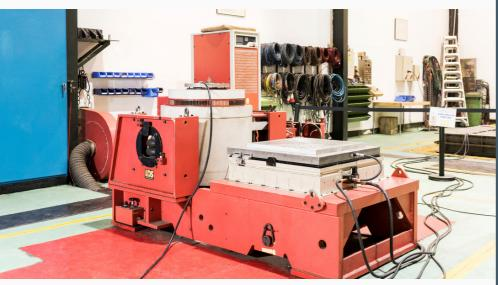
AREA OF USE: 750x750 mm ACTUATOR: Generator of 27 kN AMPLITUDE: + 19 mm MAXIMUM SPEED: 1.500 mm/s
