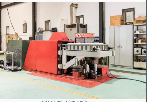
AREA OF USE: 1,200x1,200 mm ACTUATORS: 2 cylinders 100 kN AMPLITUDE: ± 125 mm MAXIMUM SPEED: 1.000 mm/s MAXIMUM ACCELERATION: 10 g FREOUENCY RANGE: 0.1 to 150 Hz
