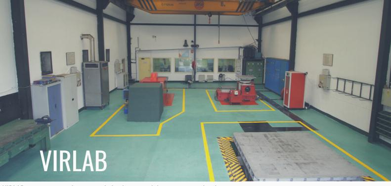
VIRLAB is a seismic, vibration and shock testing laboratory accredited by ENAC in accordance with the UNE-EN ISO/IEC 17025 standard. It is the only national laboratory approved by the Spanish Nuclear Power Plant Owners Group to carry out seismic qualification tests.
